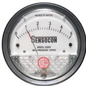
**Pressure Limits:** -20" Hg to 15 PSI (-0.677 bar to 1.034 bar)
